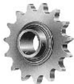
**Ready Sprockets** are an assortment of sprockets and hubs drilled and tapped for simple, convenient assembly with standard hex head cap screws. For No. 35 through No. 100 Chain, with stock finished bore hubs to accommodate shaft sizes through 2 $\frac{3}{4}$ " diameter, plus a variety of square, hex, spline, and tapered key bores.
